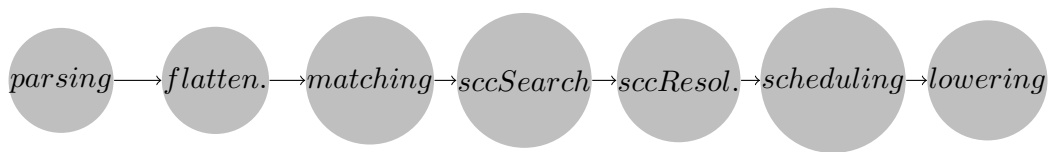
Figure 2.1: Pipeline structure of a classical Modelica compiler, comprising of several different successive stages.
