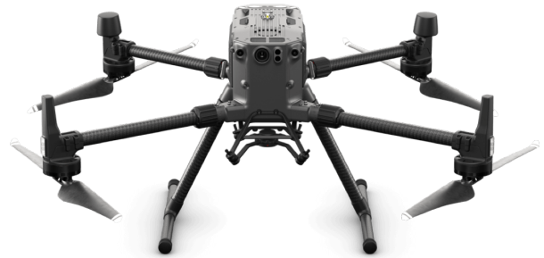
Figure 3.2: DJI Matrice 300 RTX from [63]
