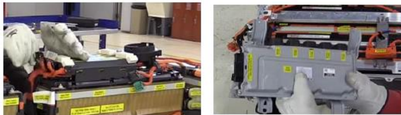
Figure 2.23: BMS removal from a battery pack
