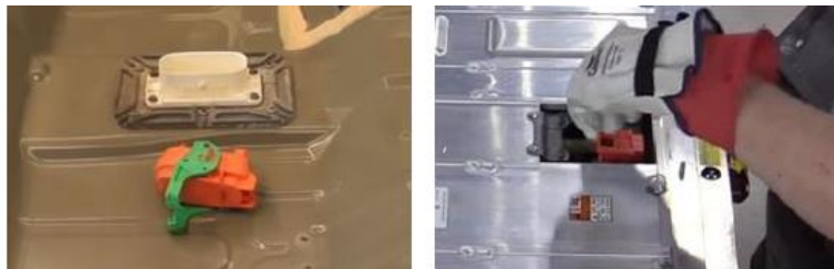
Figure 2.21: Service plug removal from a battery pack
