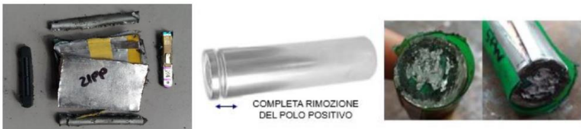
Figure 2.30: Preliminary case removal (left, prismatic; right, cylindrical)
