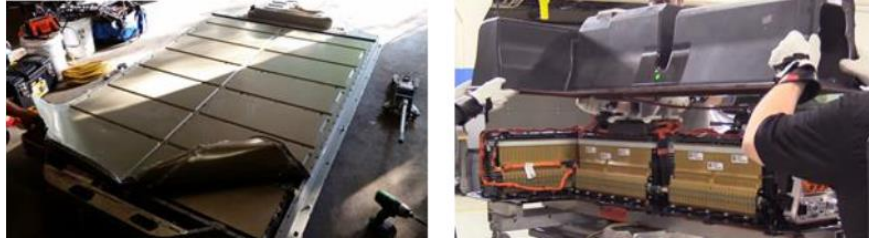
Figure 2.19: Covers removal from a battery pack
