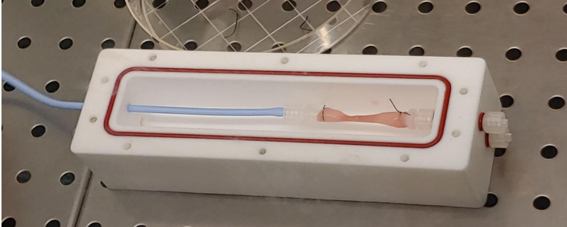
Figure 23: The oesophagus sutured at both ends in the bioreactor, prior to the application of other fittings and to connection of the chamber with the rest of perfusion system
