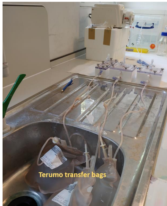
Figure 13: Further trial of hydraulic tightness (together with other two tracheal tissue engineering bioreactors). The outflow is collected in transfer bags able to exert a negative pressure inside the chamber, increasing the possibility of leakage
