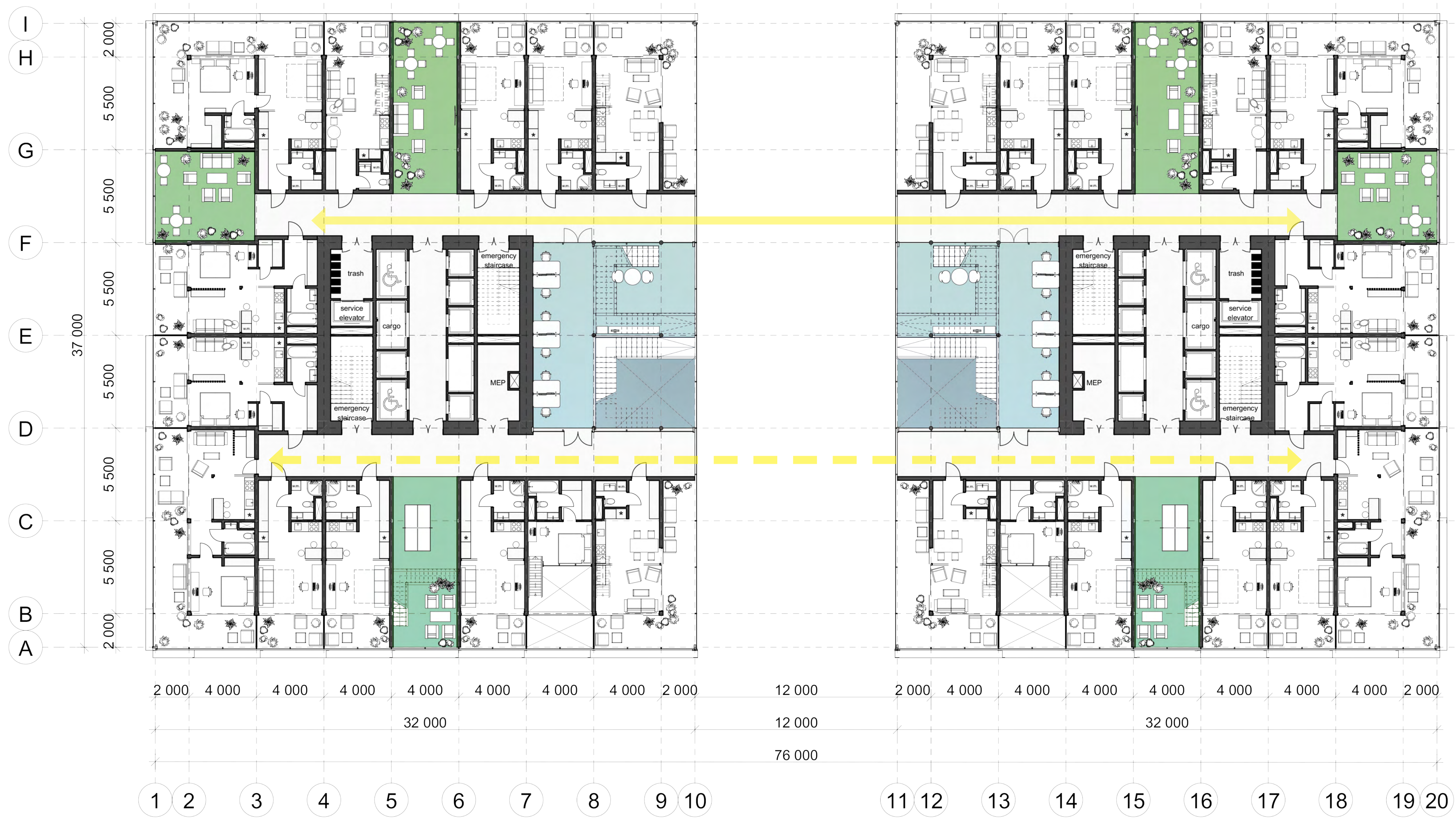
typical floor plan in a 4-level block: level 3 scale 1:150
