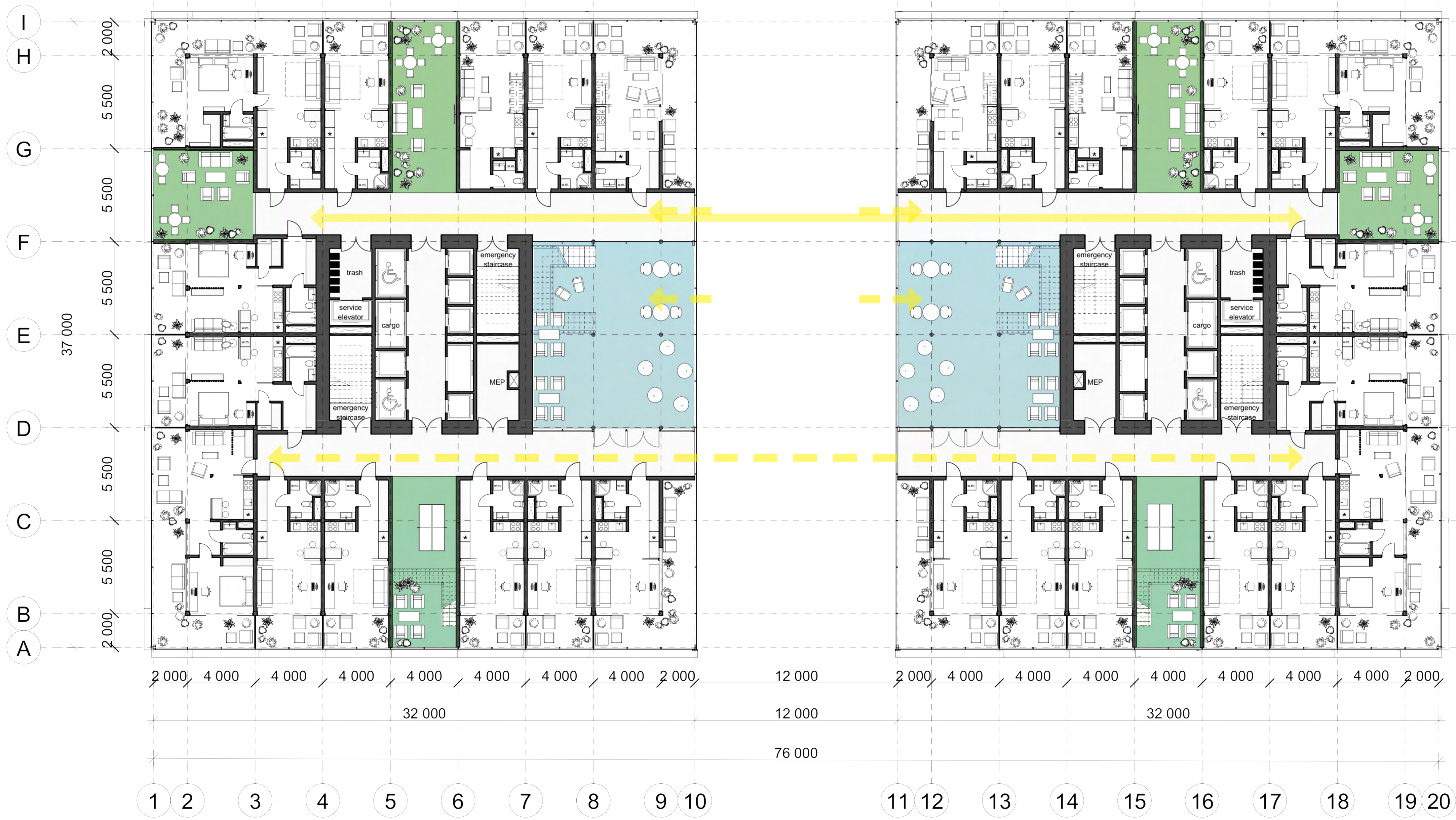
typical floor plan in a 4-level block: level 1 scale 1:150
