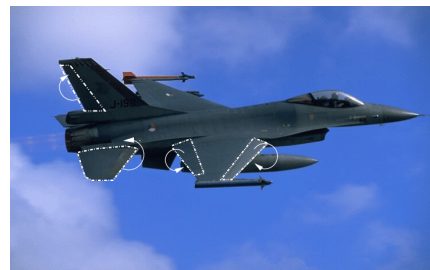
Figure 3: Main aircraft control surfaces and their typical deflection directions.
