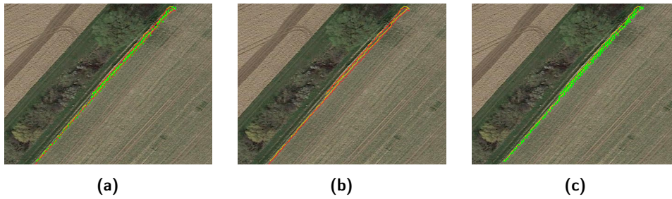
Figure 6.9: Mapviz visualization of optimized merged_bags (bag 1 + bag 2 ) in test case a. a shows the ground truth in red, the optimized robot trajectory in yellow and the landmarks (crops) in green. b shows only the ground truth and the optimized trajectories and c shows the trajectory with landmarks.
