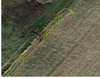
Figure 6.12: Zoomed mapviz visualization of the optimized trajectory in merged_bags on the robot turn, where it also changes the tracked crop row. We observe the optimized trajectory in yellow, the ground truth trajectory in red, the GPS measurement in blue and the landmarks as green dots.
