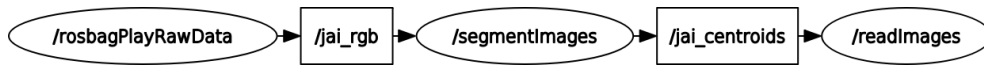
Figure 5.5: ROS nodes handling the centroids extraction. Nodes are represented as circles, while topics are inserted inside rectangles connecting a pair of nodes.
