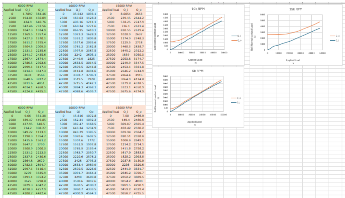
Figure 5. 2: A screenshot of the data page from the Excel file displaying the results for contact angles and normal loads
