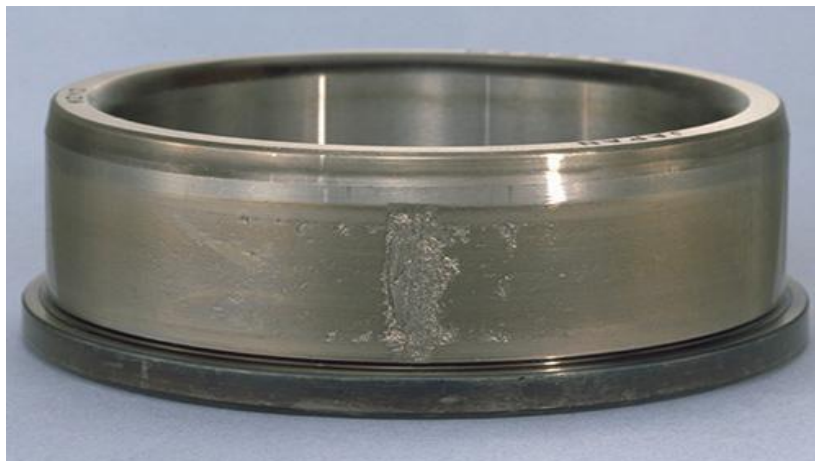
Figure 3. 10: A typical fatigue failure in a ball bearing raceway [44]
