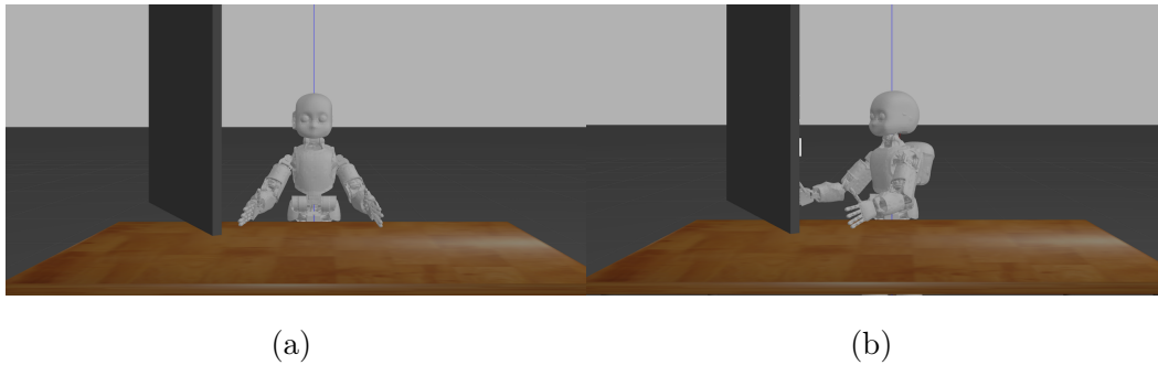
Figure 5.4: The images show the two positions, (a) the initial one with when iCub is loaded that is the home position with enlarged arms, and the second one (b) represents the robot after the rotation to reach the correct position to start the analysis.
