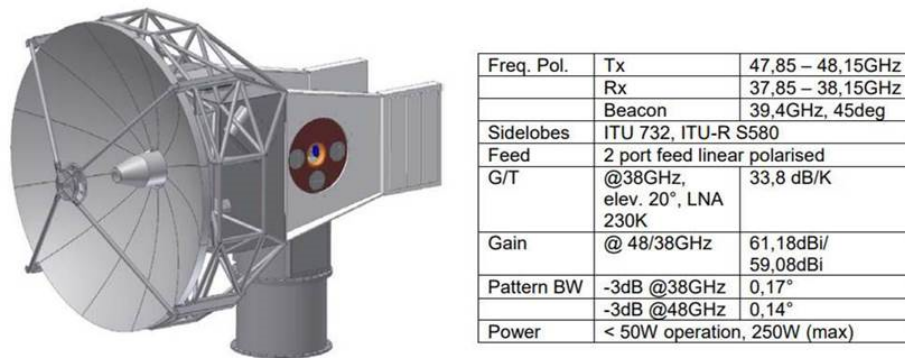
Figure 4.1: On the left CAD drawing of the 3m Q/V band antenna ©CPI Vertex Antennentechnik GmbH and on the right its specifications.
