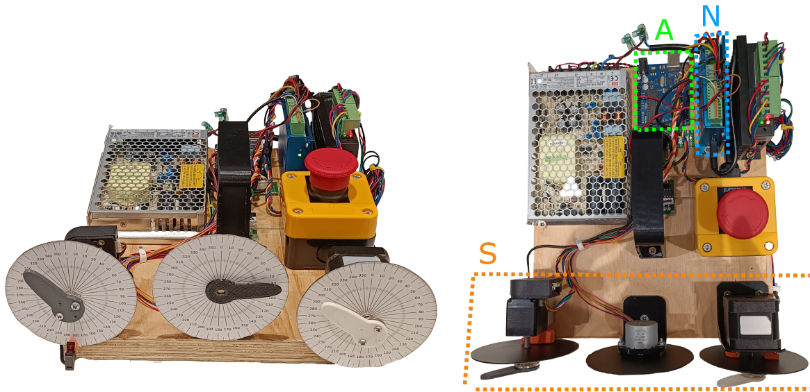
Figure 3.1: Test-bench setup - On the left, frontal view of the testbench with position indicators of the motors. On the right: top view of the testbench, with the components highlighted: A Arduino driver; N nanotec driver; S steppers
