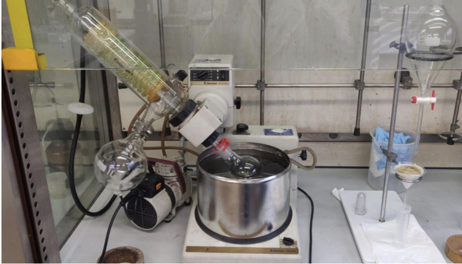
Figure 3.4 - On the left the laboratory rotary evaporator "Heidolph VV 2000" while on the right the separatory funnel of 2 L.
