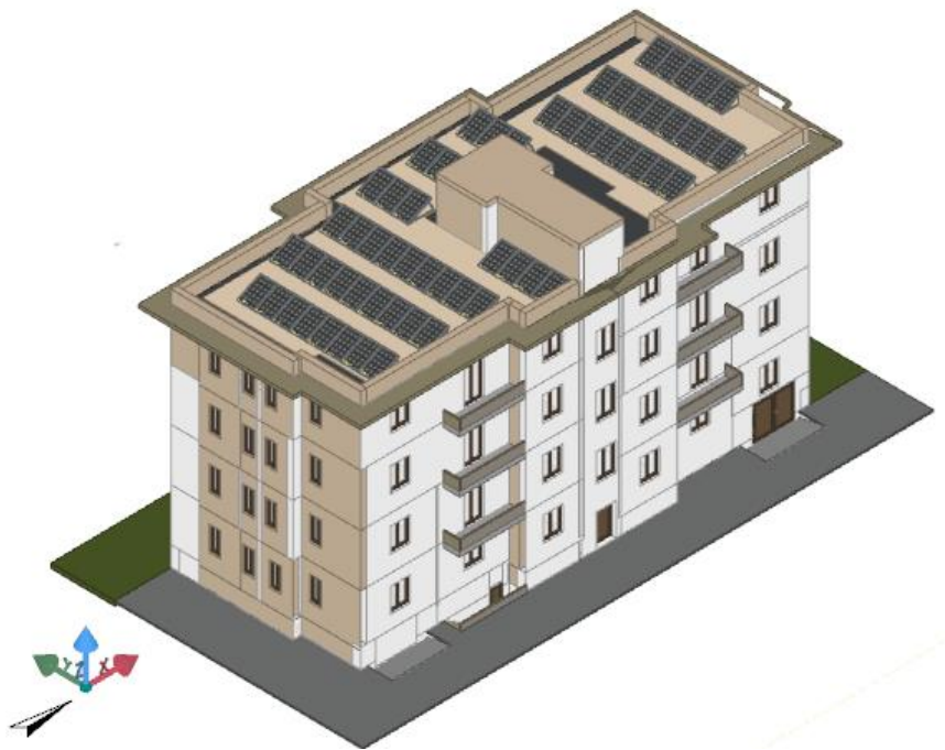
Figure 5-9 - Panel layout of Pampuri's Building
