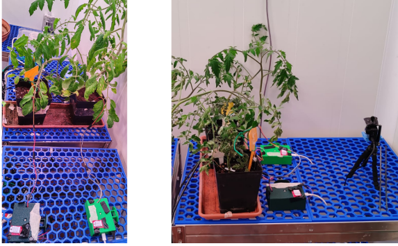
Figure 5: IMEM Parma experimental setup: Bioristor OECT electrodes implanted in tomato stems alongside Smart Plants sensor nodes.
