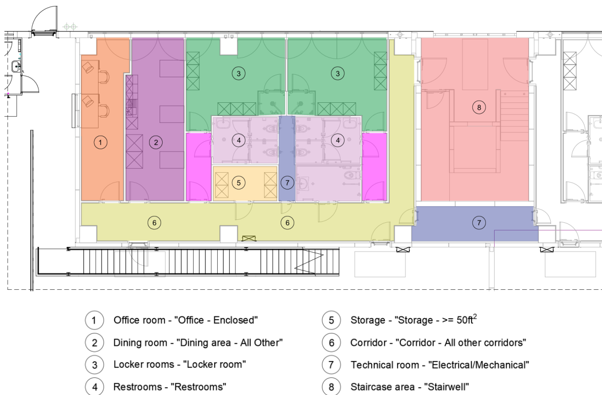
Figure 25: Scheme of the Space type assignment – example for one office block of the ground floor.
