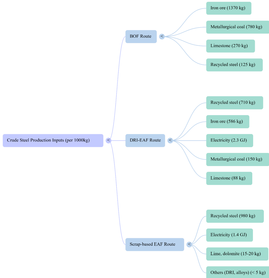
Figure 50: Three main routes of steel production and their related inputs, global average.
