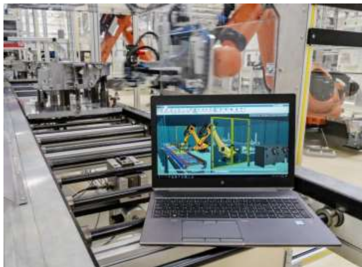
Figure 12: Digital Twin application in a production line [69].
