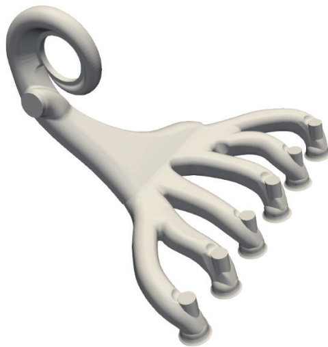
Figure 3.5 - Exhaust manifold's Standard Tessellation Language object (STL) of the engine under examination.
