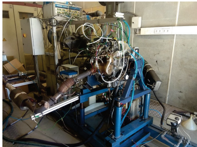
Figure 4.1 - Experimental operating points (left) and instrumented engine on the test bench (right), courtesy of UPV-CMT.
