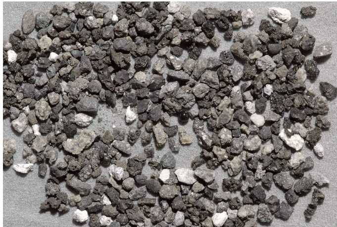
Figure 1.1: Detail of lunar regolith grains: angular, irregular fragments resulting from impact crushing processes.
