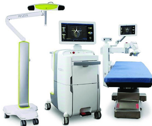
Figure 1.2: Mazor X stealth edition platform. Navigation tracking camera (left), the base station (middle), bed-mounted robotic arm with end effector (right)[12]
