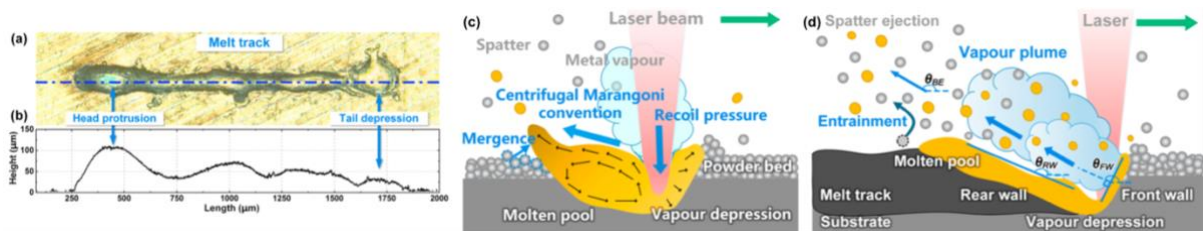
Figure 2.19: (a) Melt track morphology and (b) longitudinal profile, (c) protrusion mechanism, (d) depression zone formation (Yin et al., 2020)
