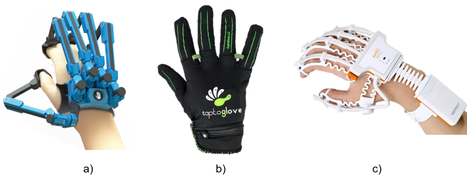
Figure 1.5: Examples of sensorized mechanical gloves. (a) Exoskeleton: SensGlove DK. (b) Fabric: CaptoGlove. (c) Striped: Rapael.
