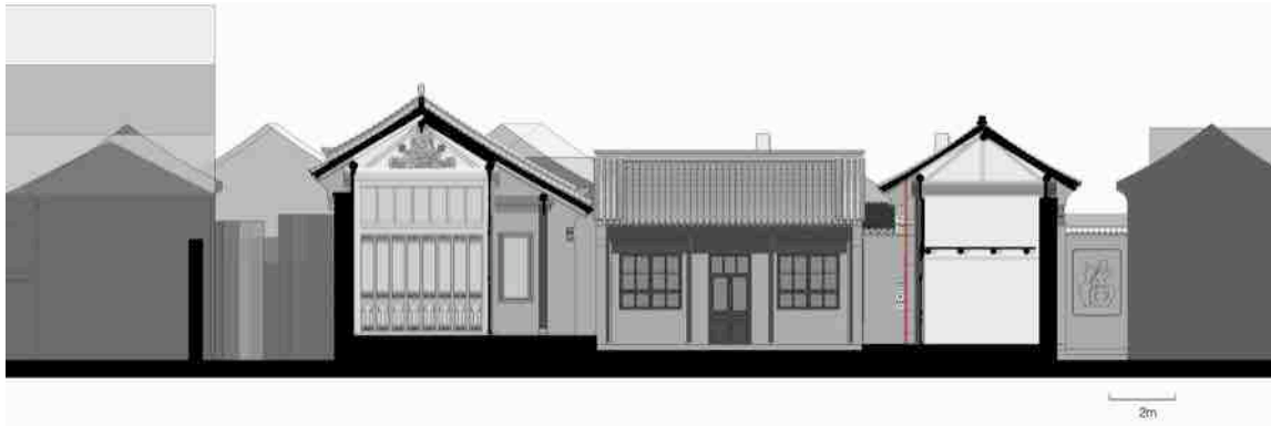
Figure 3-111 The height ratio between the attic floor and the ground floor of the building in the courtyard "Jing Shu Di." in Zhangdaicun Village. Source: Elaborated by the author.
