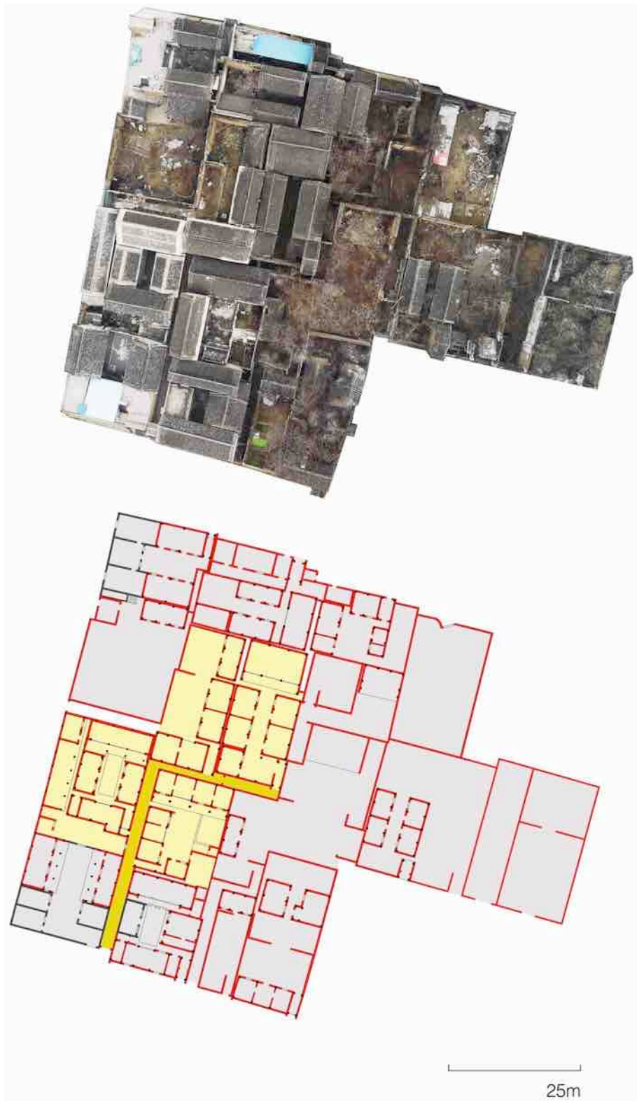
Figure 3-102 Typological diagram of Building Structure of the semantic unit A-3. This semantic unit is a cluster of the first branch of the Zhang family. The courtyards in the group are connected by a lane, and there are small doors between adjacent courtyards to connect each other. Source: Elaborated by the author.
