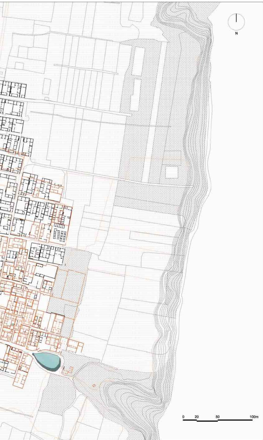
Figure 3-89 The superimposition plan of Zhangdaicun Village, plan of the 1960s and current.
