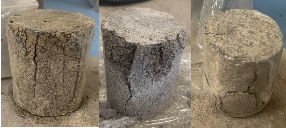
Figure 28: fracture patterns as observed during testing (Types 3/5/6 and 2)
