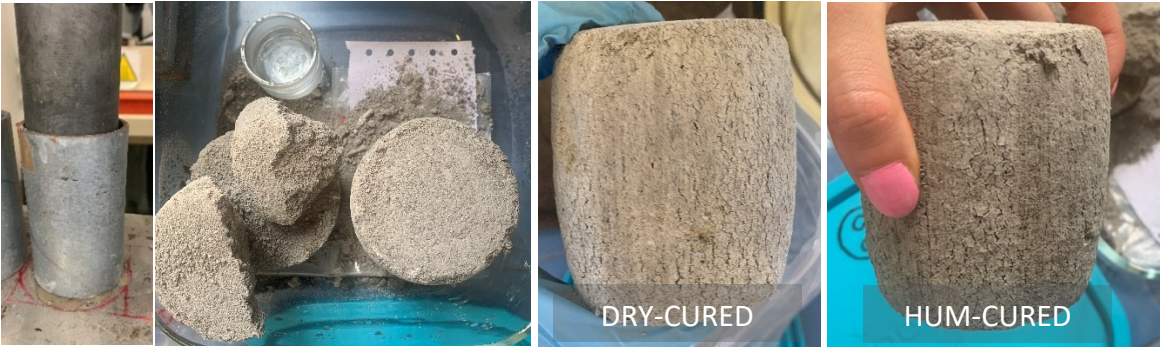
Figure 17: casting and curing of specimen
