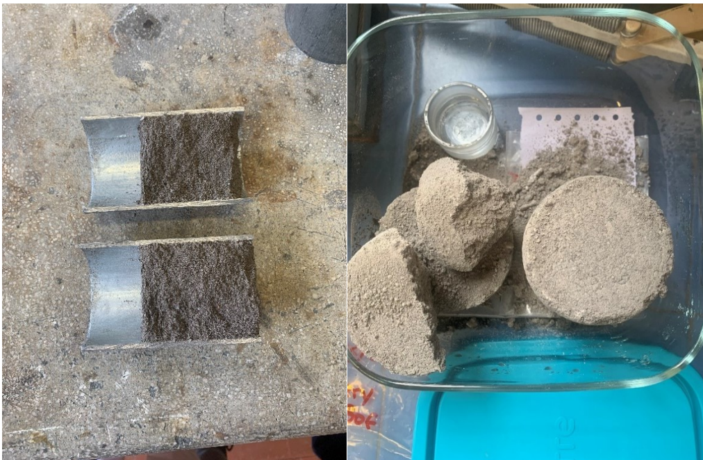
Figure 11: failed demoulding and high humidity curing attempts
