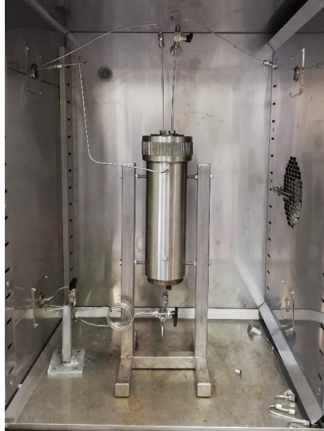
Figure 3.7: Core positioning in the oven.
