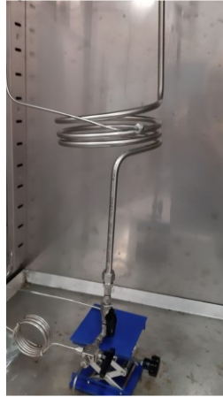
Figure 3.11: Coiled slim tube inside the oven.
