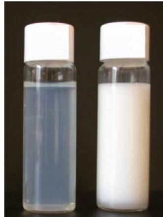
Figure 2.7: Nanoemulsion (left) and macroemulsion (right) with droplet diameters of 35 nm and 1 \mu\text{m} , respectively [40].
