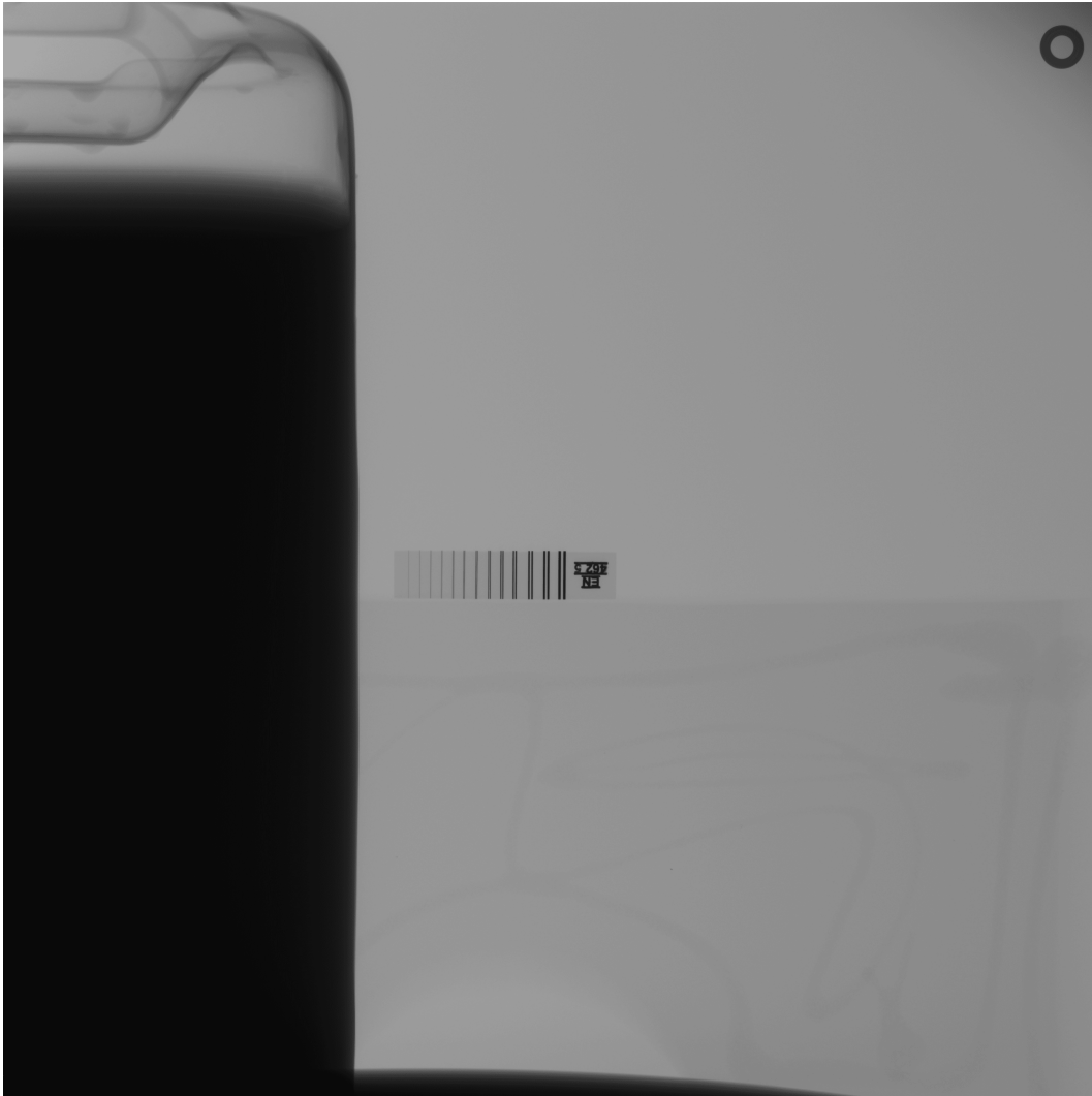
Figure 7.6: Pre filtration of 0.3 mm brass with tank near the IQI. Parameters are 180 kV, 15 mA, 90 cm SOD, M=1.17.
