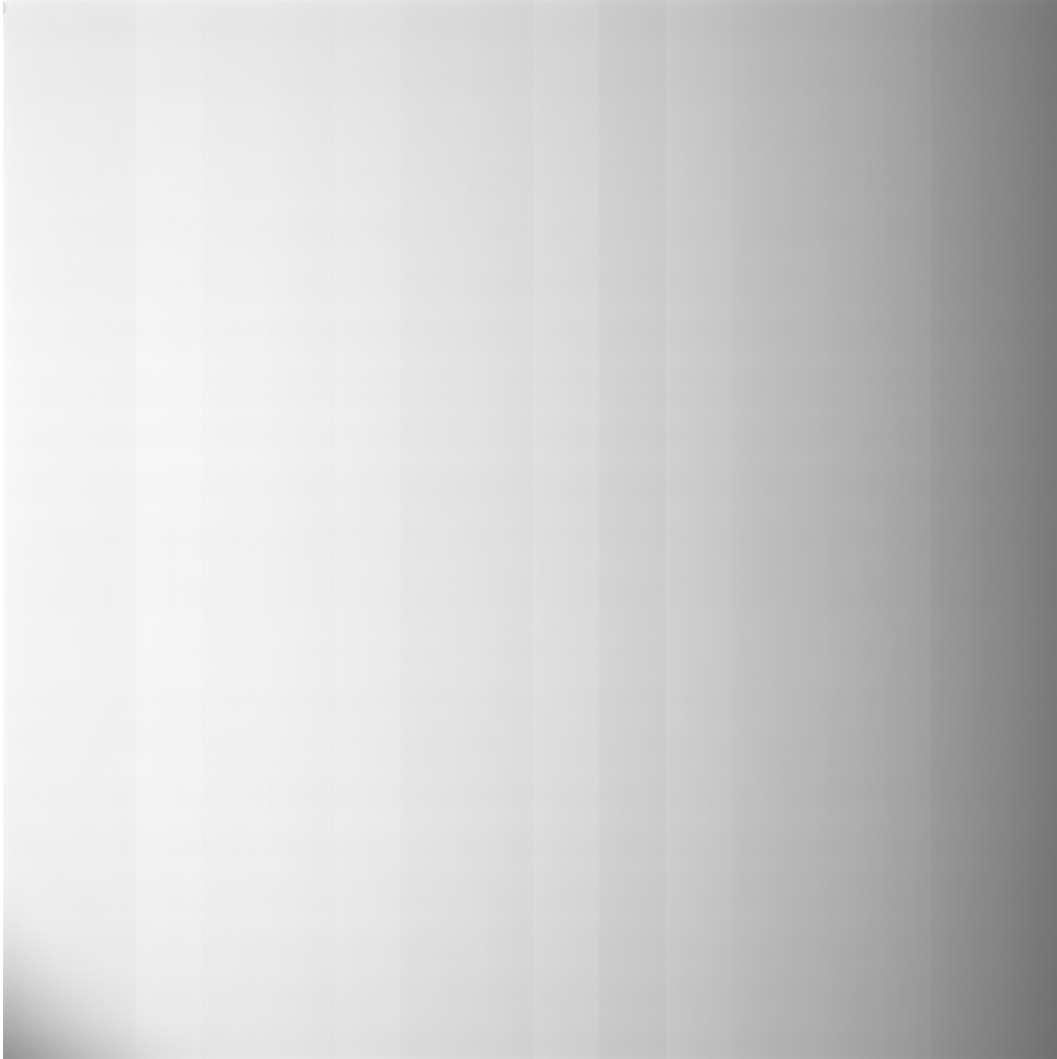
Figure 5.1: Flat field exposure without gain correction, 285 kV 3 mA 0.5 s
