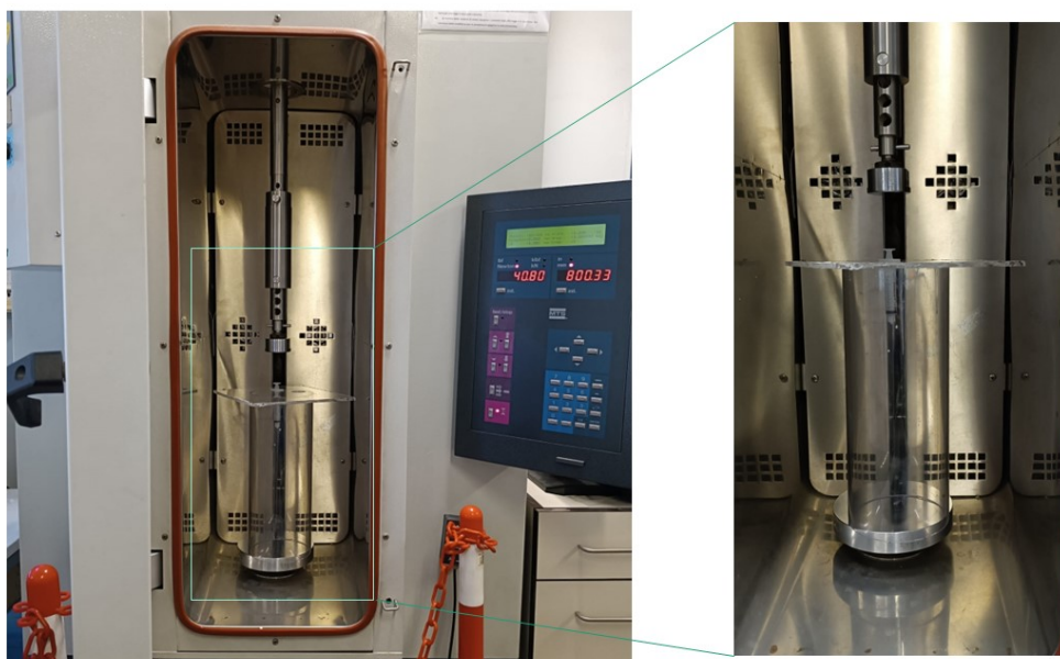
Figure 3.3: MTS electro-mechanical machine with a thermostatically controlled chamber for the injectability.
