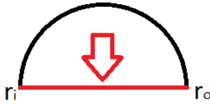
Figure 3.11: The position where the physical quantities are computed is highlighted in red, intrados r_i (left), extrados r_o (right).
