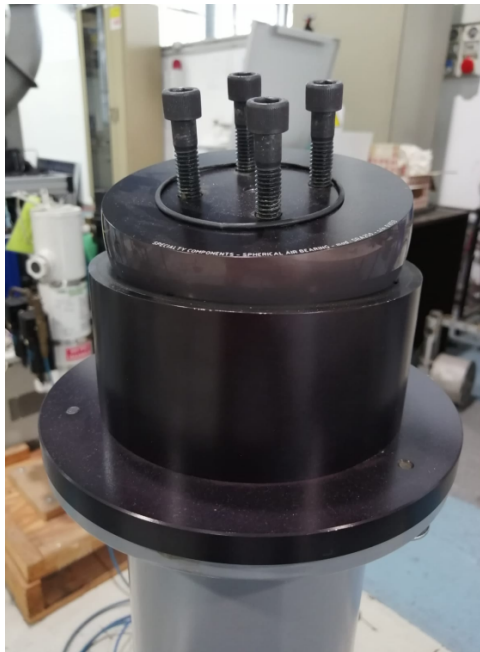
Figure 2.5: SRA250-R30 spherical air bearing
