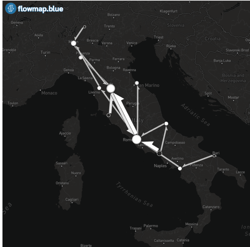
Figure 4.15. Optimal Intercity network. Fleet 200 aircrafts. Load factor = 0.8. Aircraft capacity = 19 pax. t_{\text{charge}} = 1800 s.
