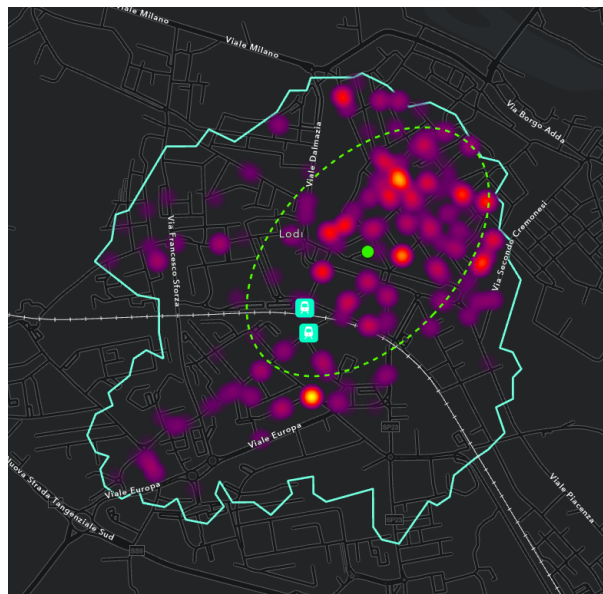
Figure 4.5: Spatial analysis carried out on Lodi station. The weighted heatmap, the services centroid and the directional ellipse are shown.
