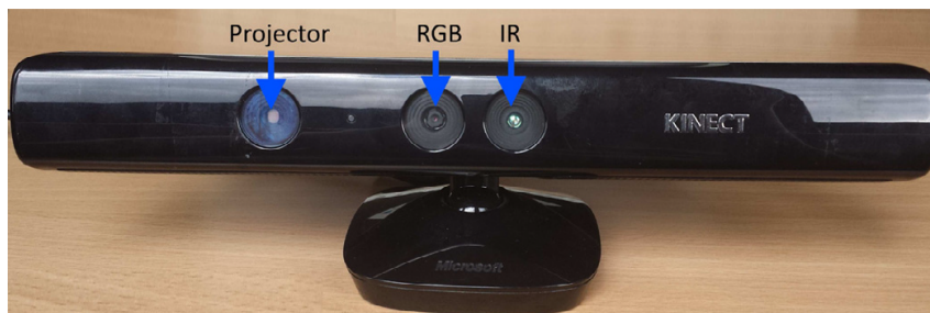
Figure 1.6: Sensor placement within a Kinect SL camera. The baseline is of approximately 7.5 cm.
