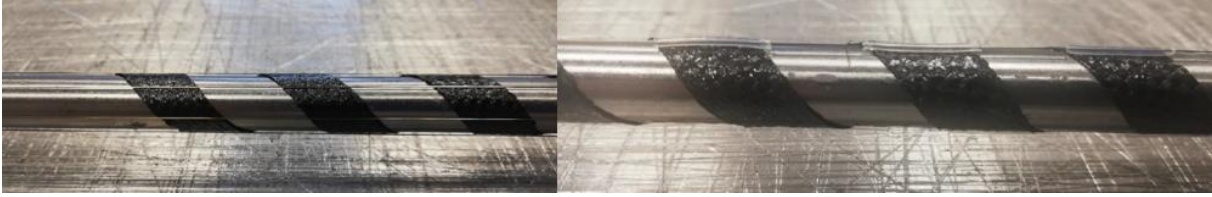
Figure 120: NiTiNOL wires directly embedded in the structure (left) and NiTiNOL wires inside sheaths embedded in the structure (right)
