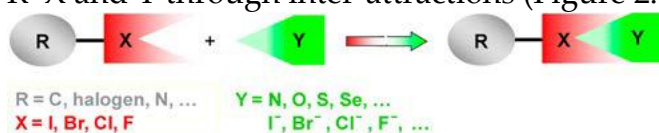
Figure 2.17. Schematic representation of halogen bond[42]
