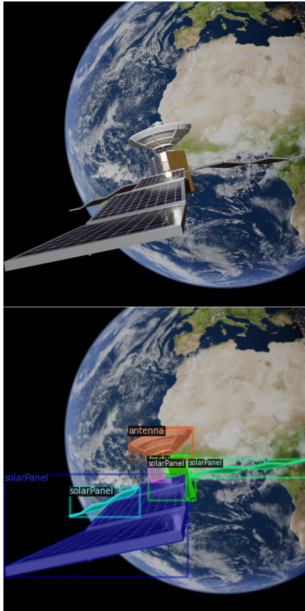
Figure 4.6: Final result of the dataset generation: the check_BB function shows the image and the ground truth masks as they were identified by the satellites_to_COCO function.
