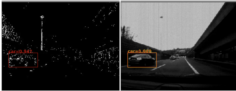
Figure 4.8: Output of the detection pipeline proposed by Chen [81]. The left image of is the DVS image with bounding boxes (in red) produced by DVS-only detection, while the right image of each pair is the APS image with DVS-only bounding boxes (in red) copied over and the RRC detections (in yellow) for comparison.
