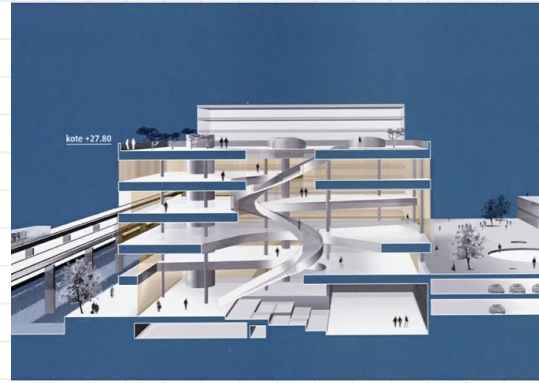
fig.18 Sistema connessione interna Ørestad Gymnasium School, Copenhagen
