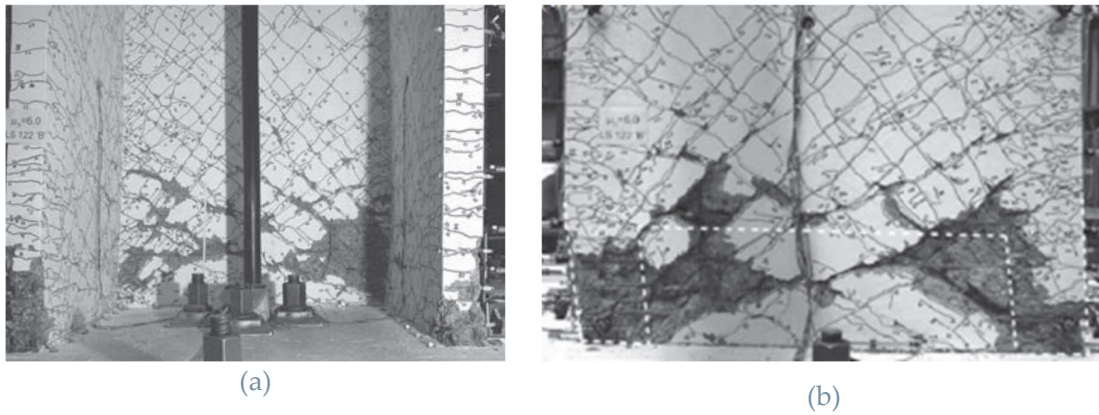
Figure 3.12 Failure of TUB (Beyer et al., 2008b)
