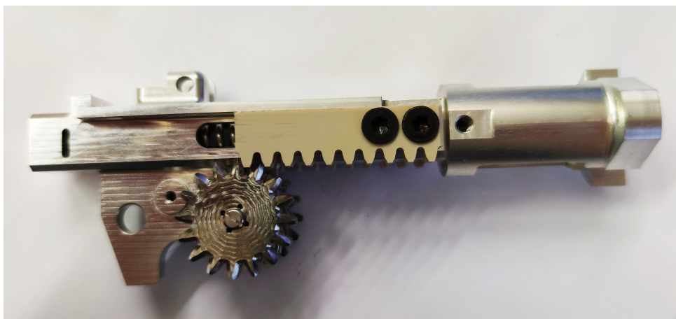
Figure 5.10: Spring loading mechanism.
