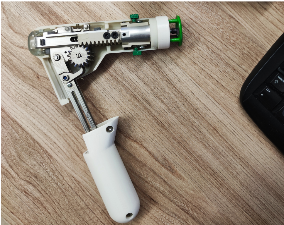
Figure 5.12: Internal mechanical components assembly completion.
