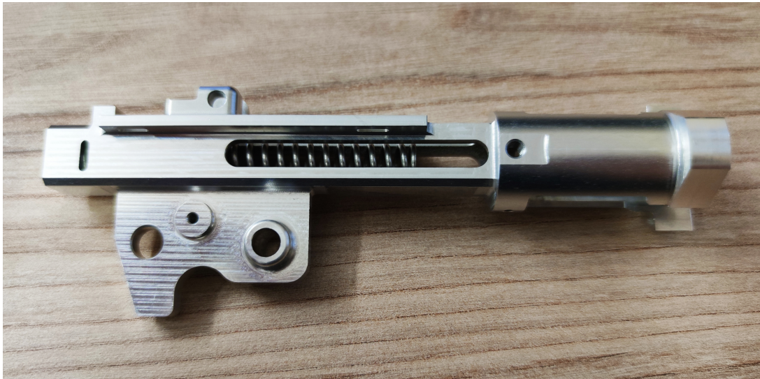
Figure 5.9: Housing body and main spring.
