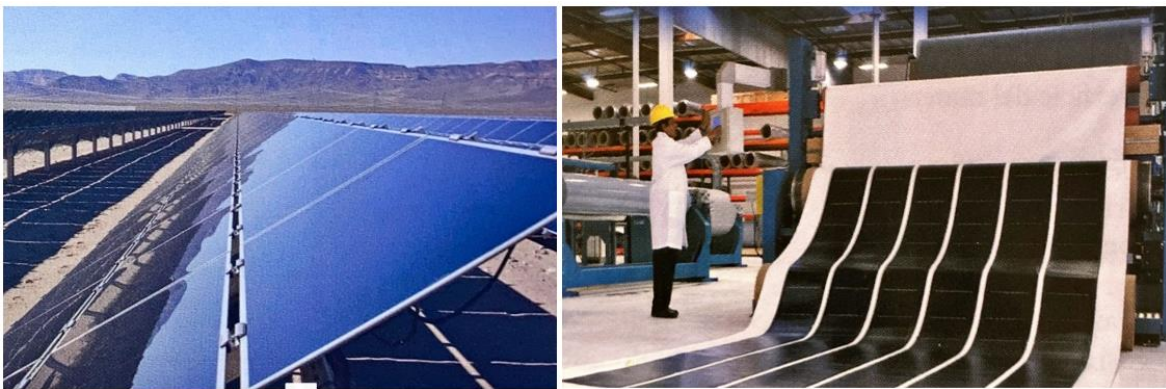
Figure 1.11: Left: CdTe thin film modules in a PV field in south western USA [4]. Right: a-Si thin film production [5].
