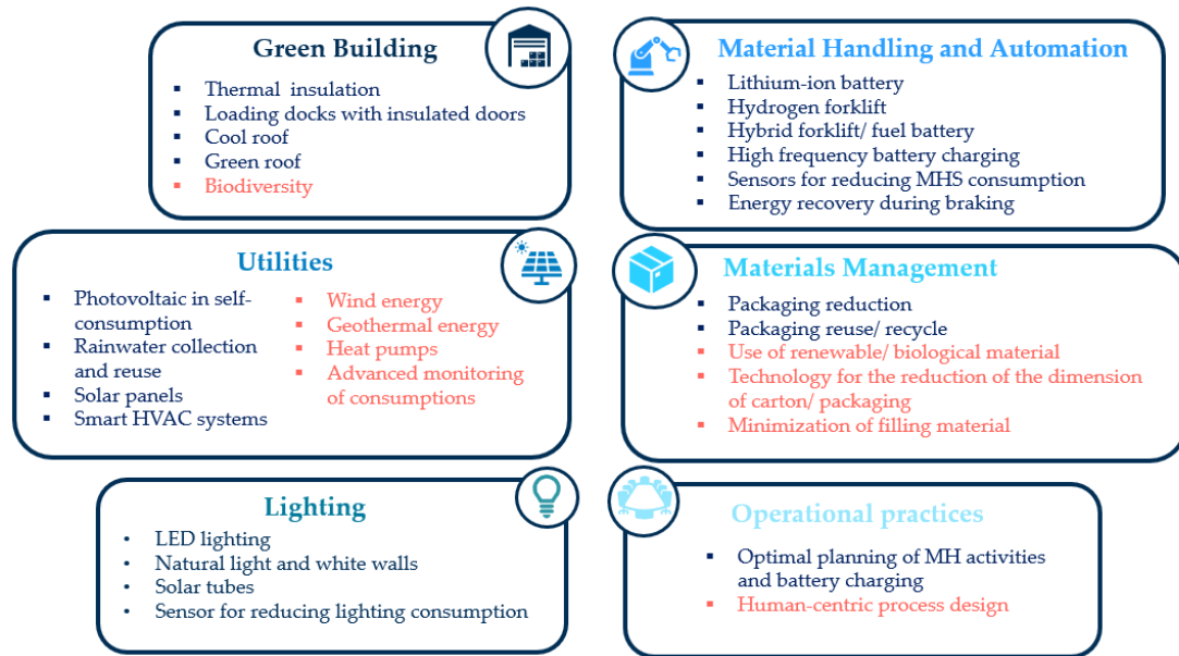
Figure 3.11 Framework of energy-efficient solutions in warehouses
