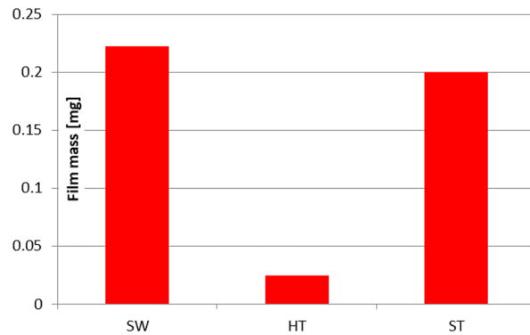
Figure 5.40: Wall film, impinged fuel mass on the piston surface, SOI 540 CA, 700 CA
