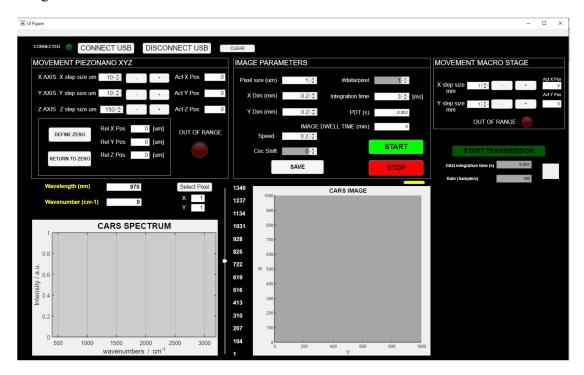
Figure 3.15: Matlab interface for the acquisition of the CARS images.
