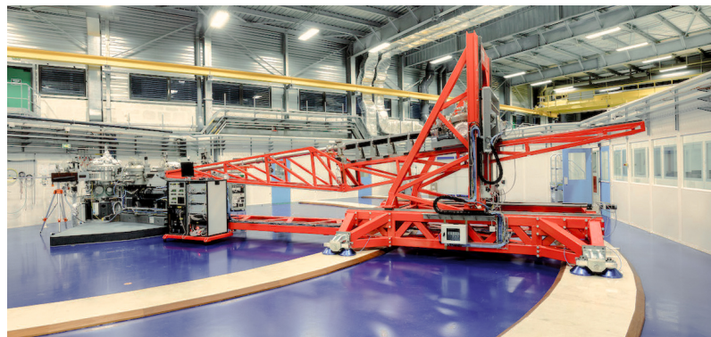
Figure 3.8: The sample chamber and the analyser of the RIXS spectrometer at ID32. Taken from [41].
