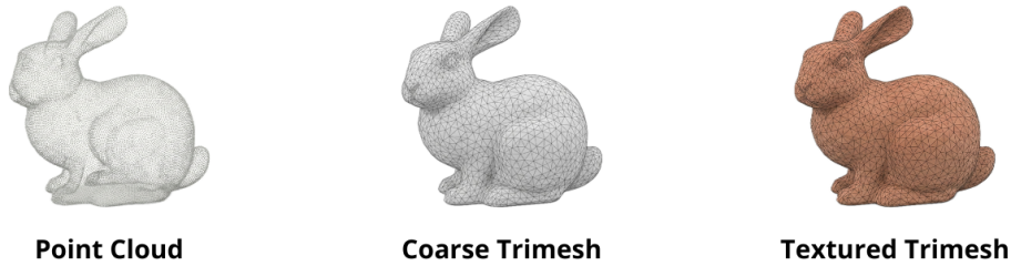
Figure 2.5: Three representations of the Stanford Bunny [48]. Left: a dense point cloud \{\mathbf{v}_i \in \mathbb{R}^3\} capturing the raw surface geometry. Center: a coarse triangle mesh \mathcal{M} with a reduced number of faces N_f , highlighting the underlying polygonal structure. Right: the same coarse mesh with a diffuse texture applied per face, illustrating how appearance information is encoded on the surface.
