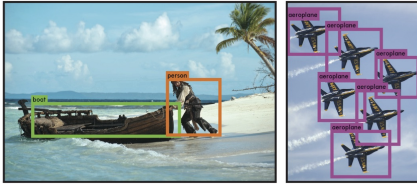
Figure 3.2: Object detection with bounding boxes and class labels using YOLO [38].
