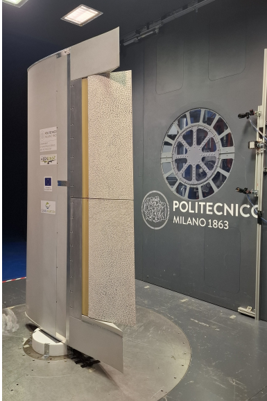
Figure 9: Morphing aileron demonstrator at minimum deflection, viewed from the pressure side.
