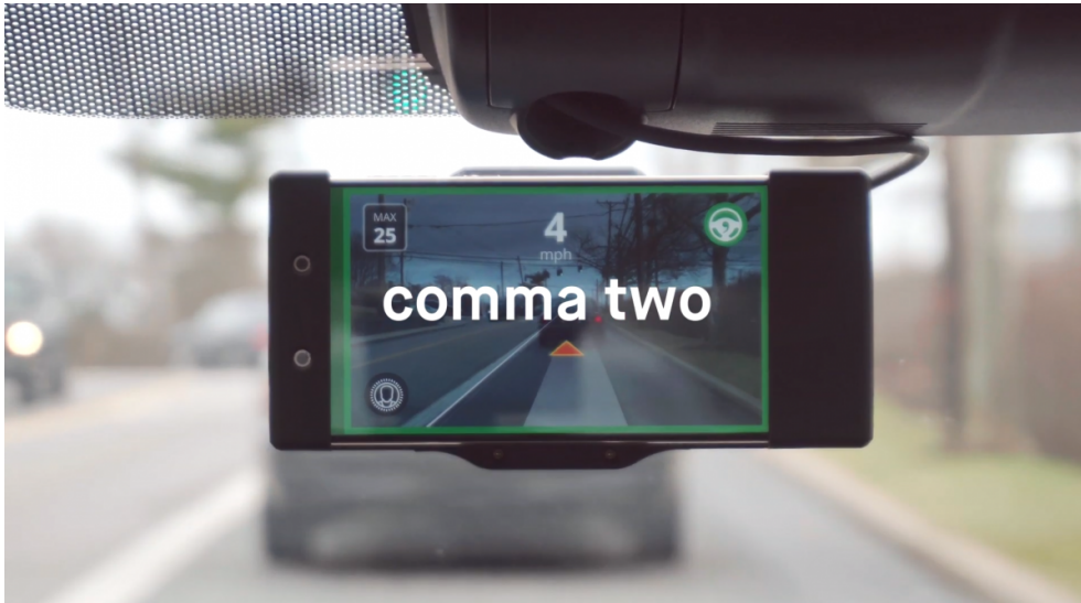
Figure 2.6: Comma.ai hardware installed on the windscreen of a compatible mass production vehicle
