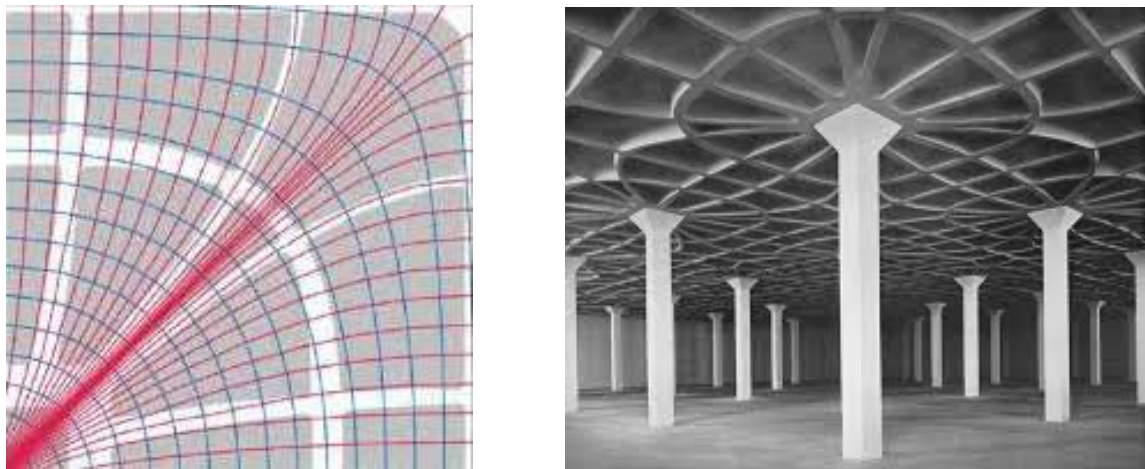
Figure 3: Principal directions of stress for a floor system and their structural application.
