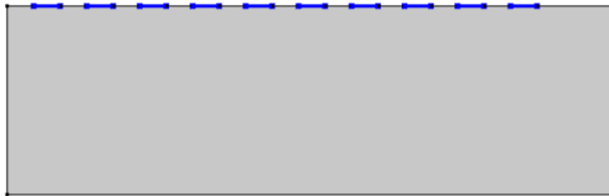
Figure 4.3: Focus on the left-side IDT. The fingers are simulated as segments placed on the top boundary of the piezoelectric substrate.
