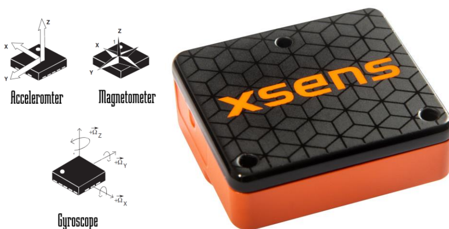
Figure 20: inertial Measurement Units (IMUs) can be considered a combination of these three devices: accelerometers, gyroscopes and magnetometers (left). An example of 9-axis IMU (Motion Tracking device) used for smartphones, tablets, wearable sensors, and other consumer markets (right).
