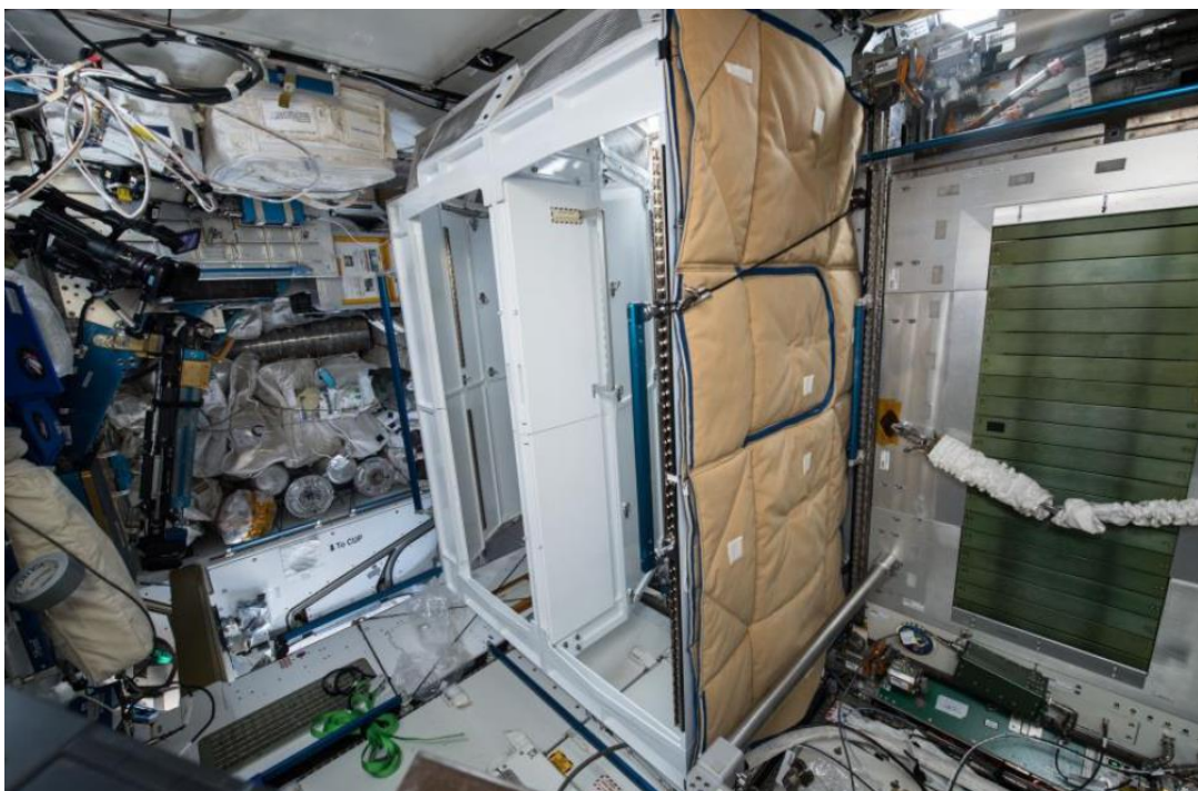
Figure 23: toilet Stall deployed in ISS Node 3 (Borrego et al., 2019). The second half of the toilet reached the ISS in October 2020. Its features and improvement will help NASA preparing for future missions, including those to the Moon and Mars.
