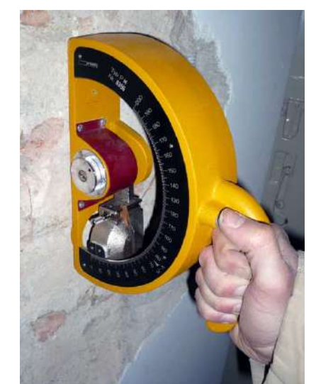
Fig. 11.4.6: Sclerometro a pendolo ( https://www.essebiweb.it/muratura2 )
